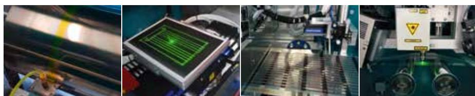
From left: Slot-die coating process, pulsed laser scribing system, inkjet printing process, in-house developed spectroscopic ellipsometry and Raman spectroscopy in-line quality control tools
