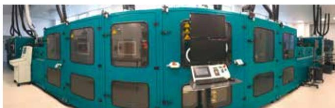
Roll-to-roll pilot production line at the COPE-H and OET facilities
